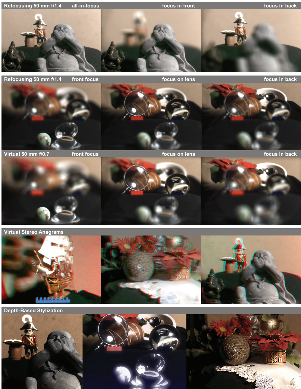
Figure 12: Examples of light-field imaging applications. Topmost row: strong refocussing with a virtual aperture matching the real Canon EF 50 mm f/1.4 USM lens, which was used to record the scene. The all-in-focus view is an example of an interpolated light-field view. Second/Third row: Refocussing in a challenging setting (specular, mirroring and refracting objects). The second row shows refocussing within the physical limits of the real aperture, the third uses extrapolation to virtually extend the aperture by one full size to each side, leading to a virtual f/0.7. This mode enables macro-photography effects for standard lenses and wide fields of view. Please, compare the quality of the in-focus regions; no significant loss in sharpness is observed for the extended aperture case, validating the suitability of our depth-estimation and view-morphing procedures. Fourth row: Virtual stereo images (in form of anaglyphs) with an adaptable base line of three light-field scenes. Fifth row: Depth-based stylization examples: from left to right, painterly/real style, bloom+contrast+coloring/real, and sharpening/blur.
