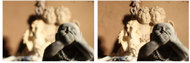
Figure 6: The aperture of the pickup system determines the depth of field of the light-field views (shown is the center view, but other views behave similarly). With open pickup aperture, depth of field effects can be clearly observed (left). With a closed pickup aperture, the views are sharply imaged over the full depth range (right).
